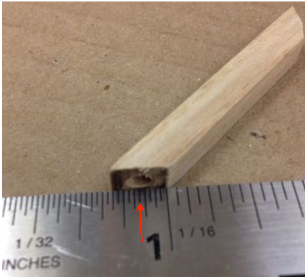
Figure 5: How to measure where to drill the guide hole.
