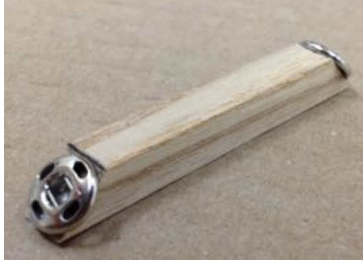
Figure 8: Trapezoid brace with snap glued in place.
