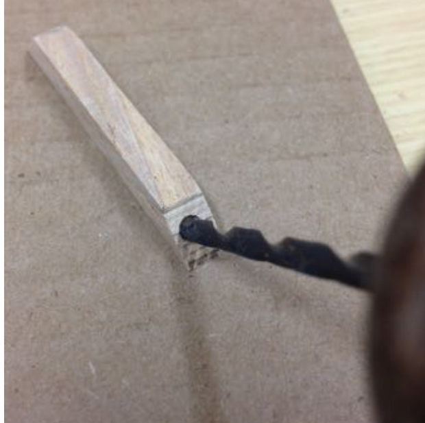
Figure 6: Drilling the guide hole in one of the shear braces.
