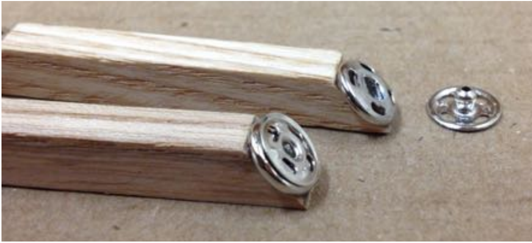
Figure 13: Place the snap base in (foreground) in order to use the diagonal brace for measurement of where to glue the bases.
