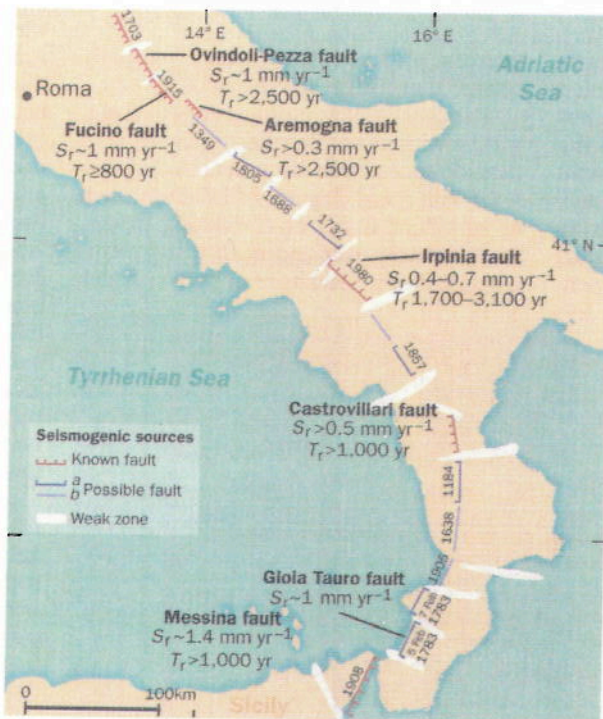
Fault segmentation, slip rate ( S_r ) and earthquake recurrence time ( T_r ) along the central and southern Apennine chain, Italy. Faults known from field observations or inferred from instrumental data are in red. Faults inferred from geological or historical data are in purple (a, high confidence level; b, low confidence). Shading marks weak zones with moderate seismogenic potential. Dates, where given, are for the last known event. (Courtesy of the Istituto Nazionale di Geofisica, Rome.)
